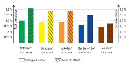
Rolling resistance is the force required to keep a wheel in uniform motion. It is influenced by wheel diameter, tread geometry, tread hardness, rebound resilience, the wheel bearing and the ground.
