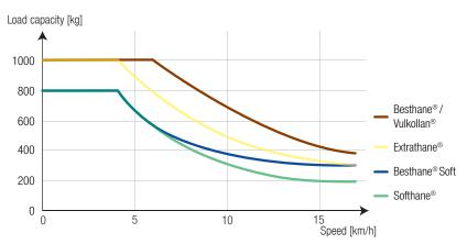
The load capacity of the tread materials decreases at higher speeds as they get hotter. The higher the rebound resilience of a material, the less the tread heats up during dynamic operation. In addition to heating, the hardness of the tread, compressive strength and ground conditions have an influence on dynamic load capacity.
