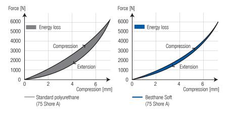
In contrast to conventional polyurethane wheels of the same hardness, Besthane® Soft wheels have a significantly higher rebound resilience, which is why the energy loss (hysteresis) during the rolling of the wheel is significantly lower (reduction of around 30 percent). Due to the reduced energy loss of the wheel, Blickle polyurethane wheels have very low rolling resistance.
